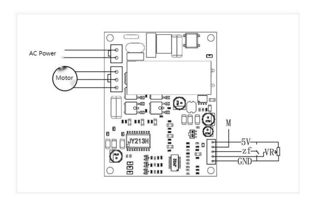
5V -----Driver board internal output voltage
